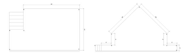
The deck on the left adds a stairway. This is pretty straight forward. The cable can go from "A" to "C" at the bottom of the stairs with one run and around the deck from "D" to "G" with another run.
